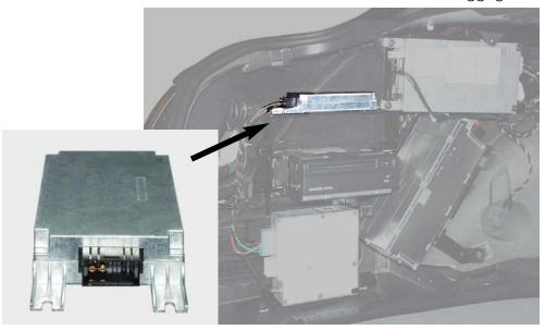
The SVS control unit has one 12 pin ELO connector that supplies KL 30, KL 31 and the two MOST connections.
